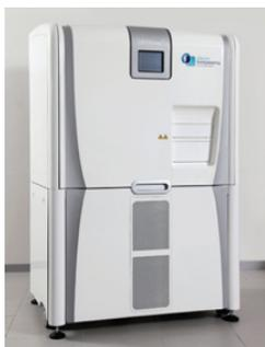
**DepArray – 2<sup>nd</sup> generation (Silicon Biosystems/SBI):** Dielectrophoretic cage capture, 6-channel IF, and single CTC recovery for DNA/RNA profiling
