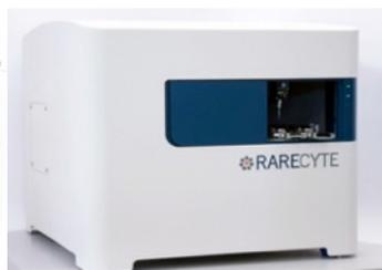
**RareCyte + Leica RX<sup>m</sup>:** Analyses all nucleated cells (no enrichment). Automated high throughput 4-channel staining (Leica) followed by high-content scanning and image analysis for CTC identification and robotic micropipette recovery (RareCyte). Use for CTC enumeration, protein and RNA -IF/FISH, and single CTC recovery for DNA/RNA profiling
